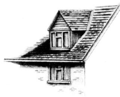
Acceptable dormer that is set into the roof and matches the windows below
